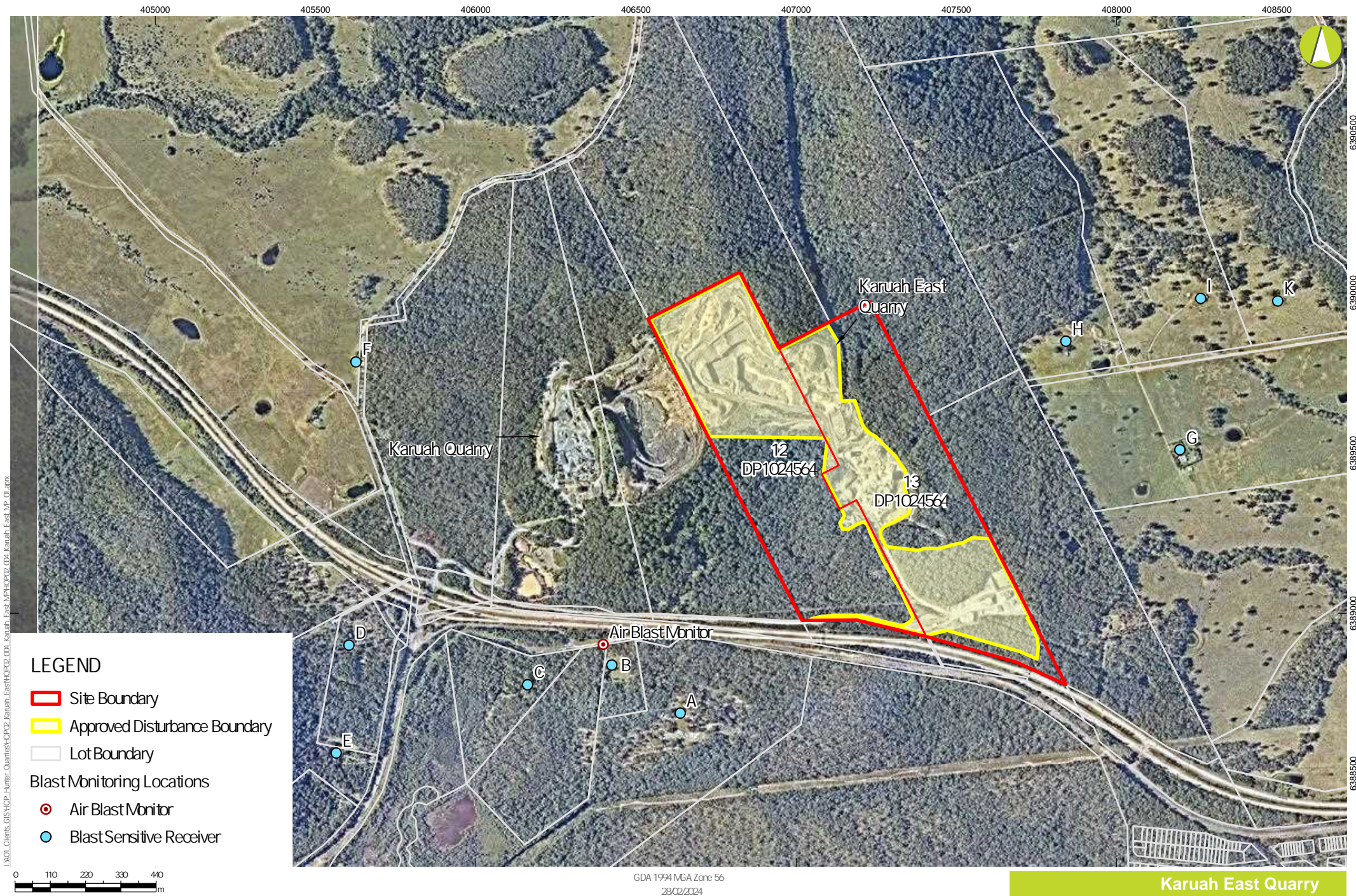
Blast Management Plan FIGURE 5 - Blast Monitoring Locations
