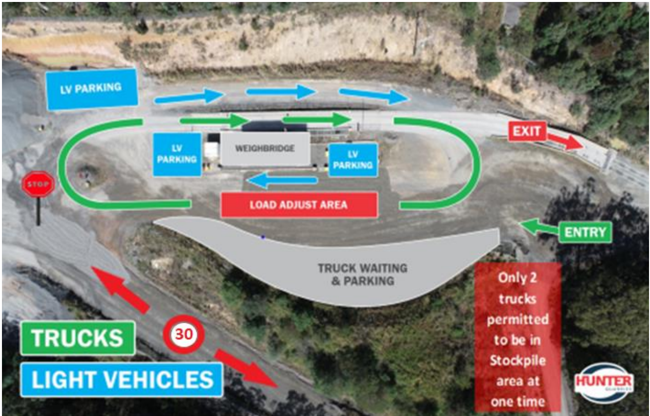
Figure 5 – Heavy Vehicle Directional Operating Rules Around the Site Entry and Weighbridge.
