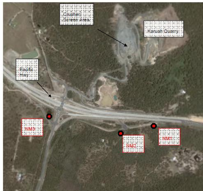
Figure 2 - Noise Monitoring Locations
