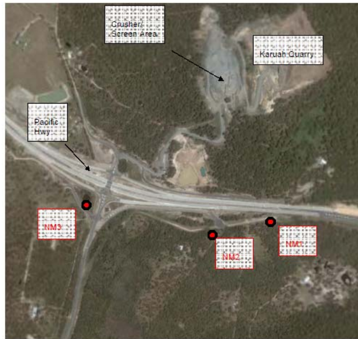
Figure 2 - Noise Monitoring Locations
