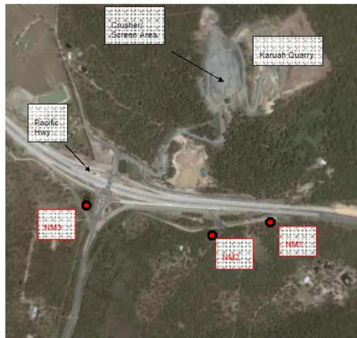
Figure 2 - Noise Monitoring Locations
